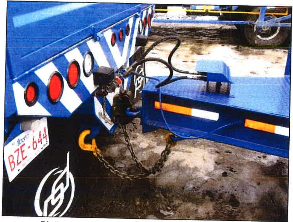
Pintle hitch & safety chains: criss cross formation
