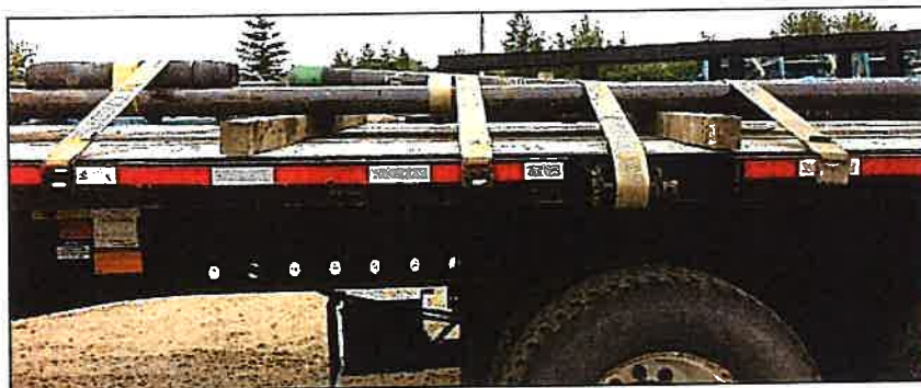
Planking w/ dunnage
