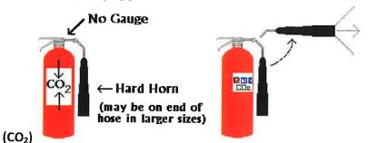
The pressure in a CO<sub>2</sub> extinguisher is so great, bits of dry ice might shoot out of the horn!
