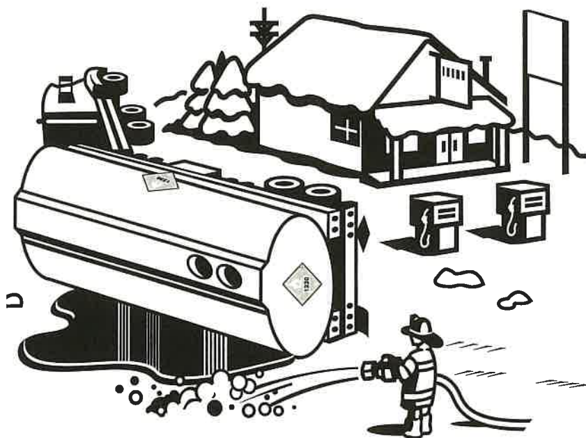
Firefighters cover the spilled methanol with foam to prevent a fire or explosion.
